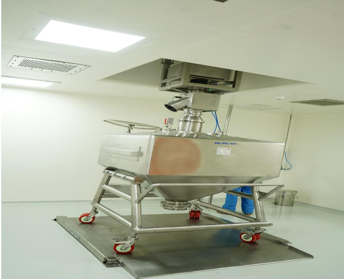
Close Loop Unloading line with Metal Detection
