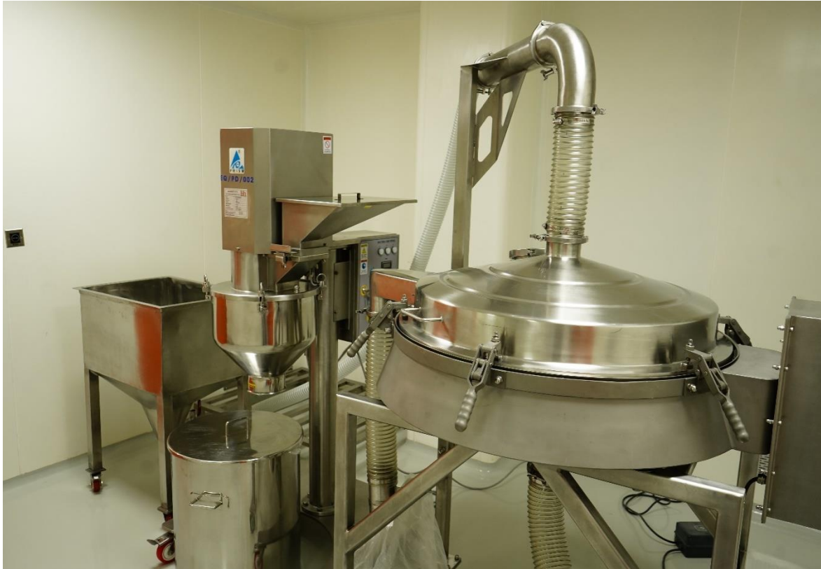
Vacuum-rated sifter with vacuum Transfer System
