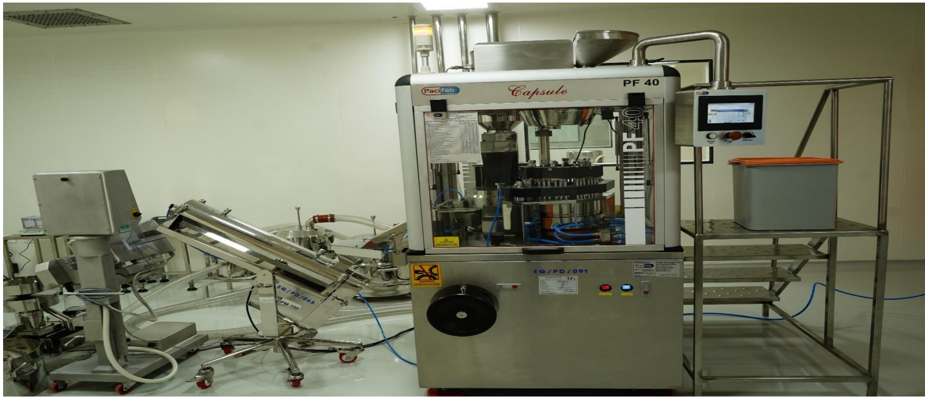
Capsule Filling Machine with online metal detection
