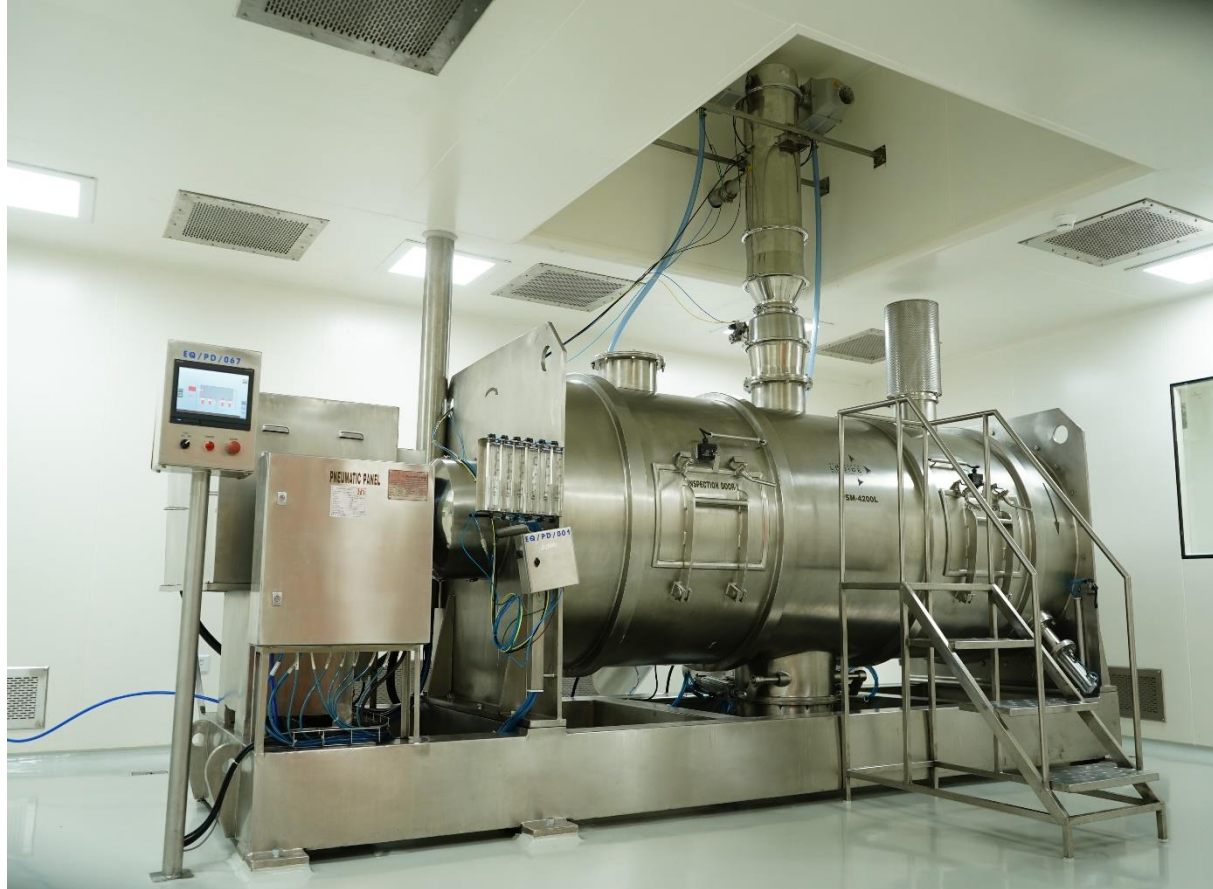
Inline Powder loading system (VTS) with Plough Mixer
