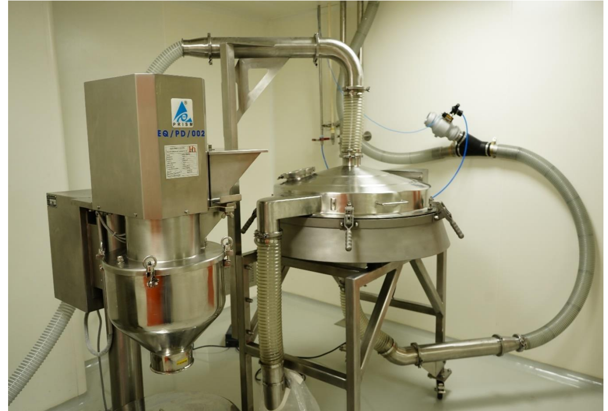
Vacuum-rated sifter with vacuum Transfer System
